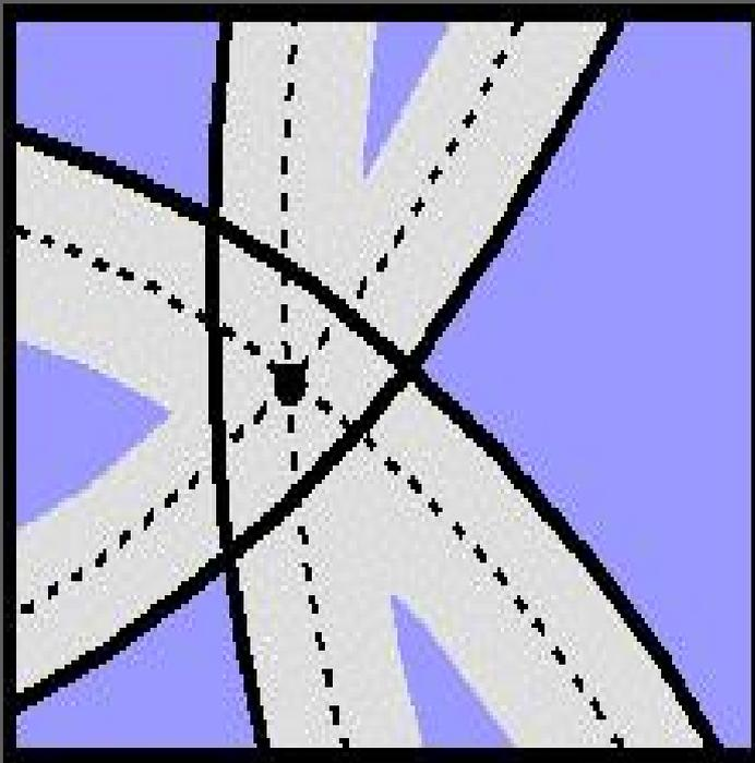
In this diagram, the solid lines indicate where the GPS receiver "thinks" the spheres are located.
