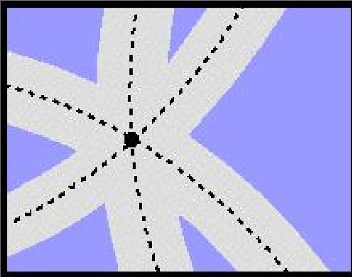
Because GPS receivers do not have atomic clocks, there is a great deal of uncertainty when measuring the size of the spheres shown in the diagram on the previous page. In the figure at left, the dashed lines show the actual intersection point, and the gray bands indicate the area of uncertainty.
