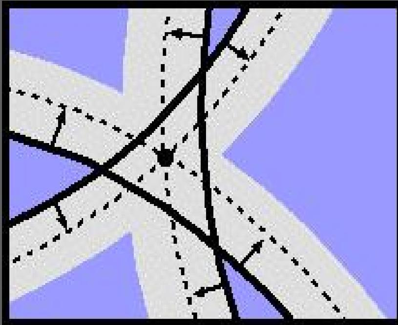
The GPS receiver must change the size of the spheres until the intersection point is determined. The relative size of each sphere has already been calculated, so if the size of one sphere is changed, the other spheres must be adjusted by **exactly the same amount**.
