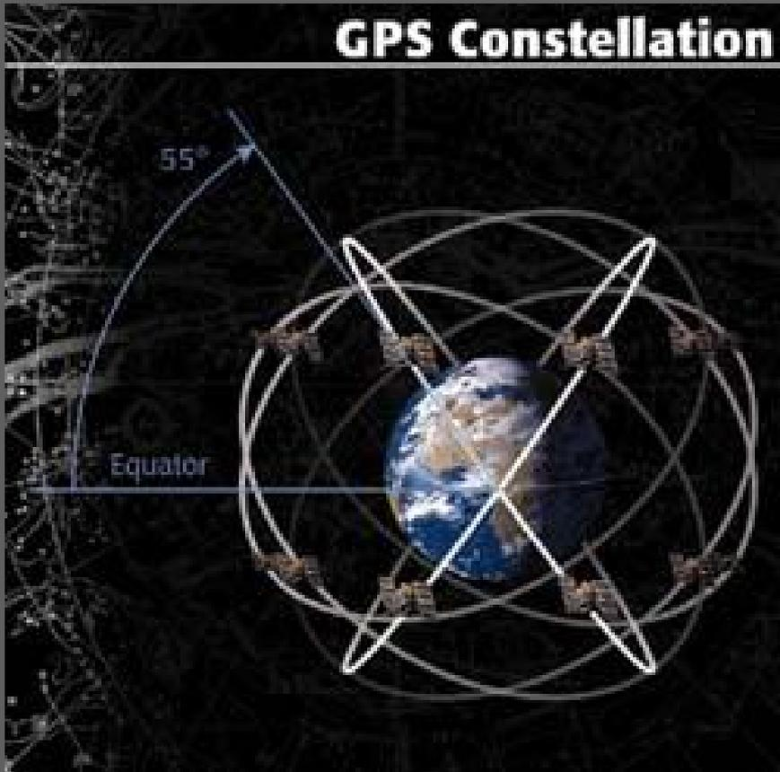
There are at least 24 operational GPS satellites at all times. The satellites orbit with a period of 12 hours.
